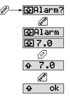
In this example the shallow water alarm is deactivated. The set alarm threshold of 7 m is stored by the unit.
